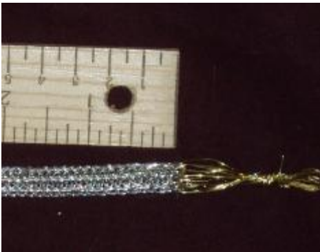
Figure 6: After being drawn the diameter was 11/32 " and the total woven length was 30.125"
